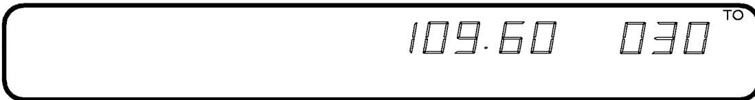
VORE MODE: ACTIVE "BEARING TO" FUNCTION DISPLAY
