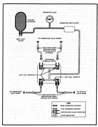
Figure 14. Oxygen System Schematic
