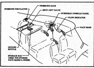
Figure 12. Oxygen System Diagram
