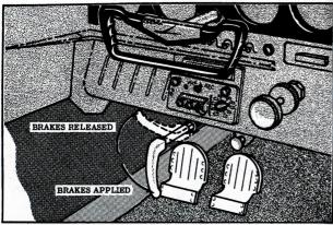
Figure 8. Parking Brake Operation
