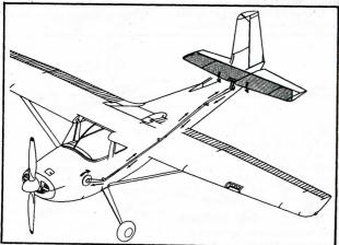
Figure 36. Adjustable Stabilizer Control System
