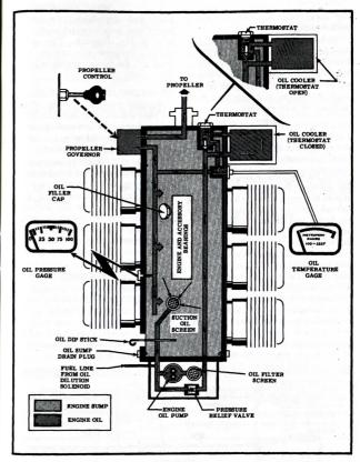
Figure 3. Oil System Schematic
