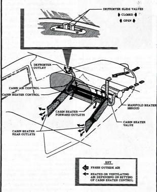
Figure 9. Cabin Air Temperature System
