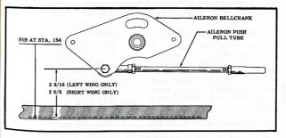
Figure 33. Aileron Bellcrank Adjustment
