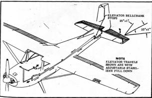
Figure 35. Elevator Control System
