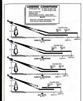
Figure 27. Water Landing Diagram (Floatplane & Amphibian)
