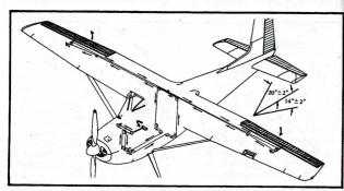
Figure 32. Aileron Control System
