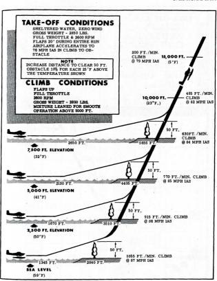
Figure 17. Water Take-Off Diagram (Floatplane & Amphibian)
