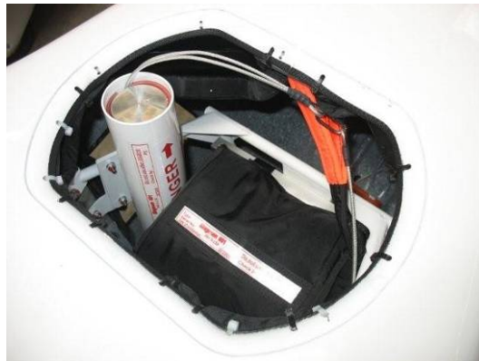
Installation of Junkers Magnum rescue system (Softpack)
