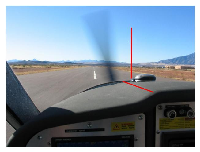
Due to the rapid curvature of the cowling and windscreen the correct longitudinal alignment is deceiving. When seated in the left seat the nose will appear as if it is well to the right of center, however this awkward visual is required to line up the longitudinal axis correctly. The centerline should look as if it is running between your feet, and the nose will look well right of centerline.
